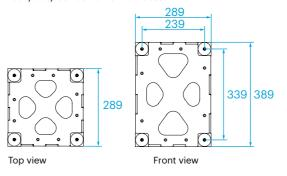
In horizontal direction the boxcorner takes the H4OR truss and in vertical direction the boxcorner takes the H3OV truss.
