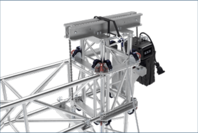
Detail of the Sleeve Block with motorised chain hoist. The span truss (QL52A) and the Sleeve Block feature a fork connection to ensure enhanced load capacity.
