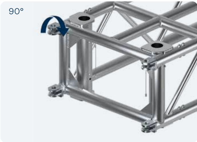
PR60TN Forks can be positioned in either vertical or horizontal orientation using a standard Allen key
