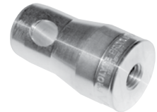
CCS6-602 weight = 0,116 kg Offset half conical coupler Offset 19 mm, thread M12
