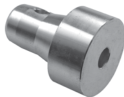
CCS6-652-23,5 weight = 0,469 kg Half conical coupler Offset 23,5 mm, 12,5 mm hole To be used with a M12 Hexagon head
